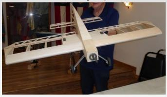
porated some improvements to the model, including formed aluminum landing gear, strengthening in the nose, and servo placement to help with balance.
