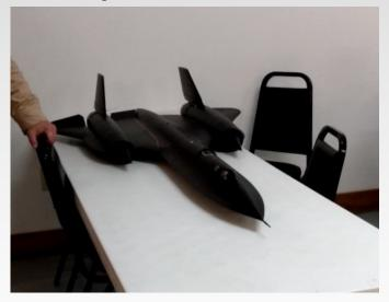
This is a large model airplane. Constructed of EDF foam, it is 74.6 inches long with a37.8 inch wing span. The empty weight is about 7.8 Lb. The
