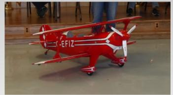
span and weight range 18 - 22 Lb. resulting in a wing loading of  $28\pm$  oz/ft<sup>2</sup>. Recommended power is 50 - 60cc gas or equivalent electric.
